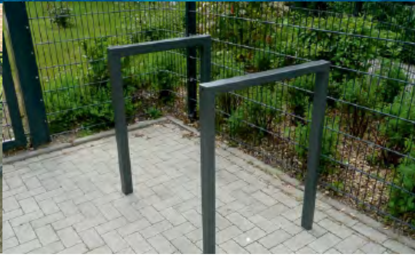
Lean-on hoop made of steel tube - for casting in concrete, Hot-dip galvanized and optionally powder-coated in DB 703. total height: approx. 1200 mm
